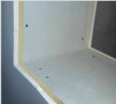
Easy visual inspection onsite. Look for the yellow core
